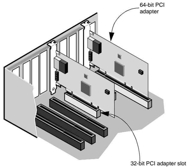
6. Push the adapter into the slot until the adapter is firmly seated. Then secure the adapter bracket with a screw.
