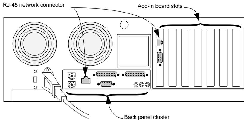
2. As shown in the figure, the network connector is an RJ-45 connector. If there is a network connector only in the back panel cluster, it is possible that the computer motherboard has a compatible LAN on motherboard (LOM) solution. Contact the motherboard manufacturer and, if it is compatible, perform the following steps:
