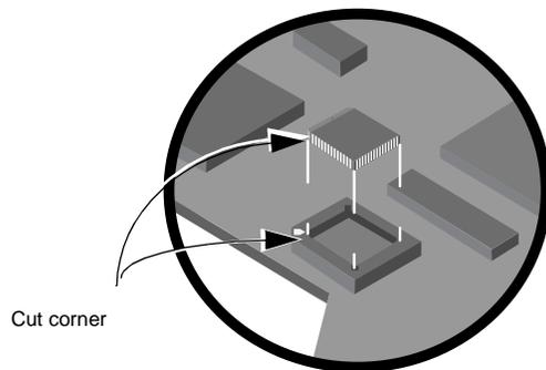
4. Refer to the figure and install the supplied flash ROM device in the socket of the adapter. Note the location of the cut corner of the flash ROM device and the corresponding cutout in the socket. There is only one correct orientation for the flash ROM device.
