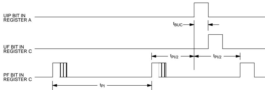
$t_{PI}$  = PERIODIC INTERRUPT TIME INTERVAL PER TABLE 1
