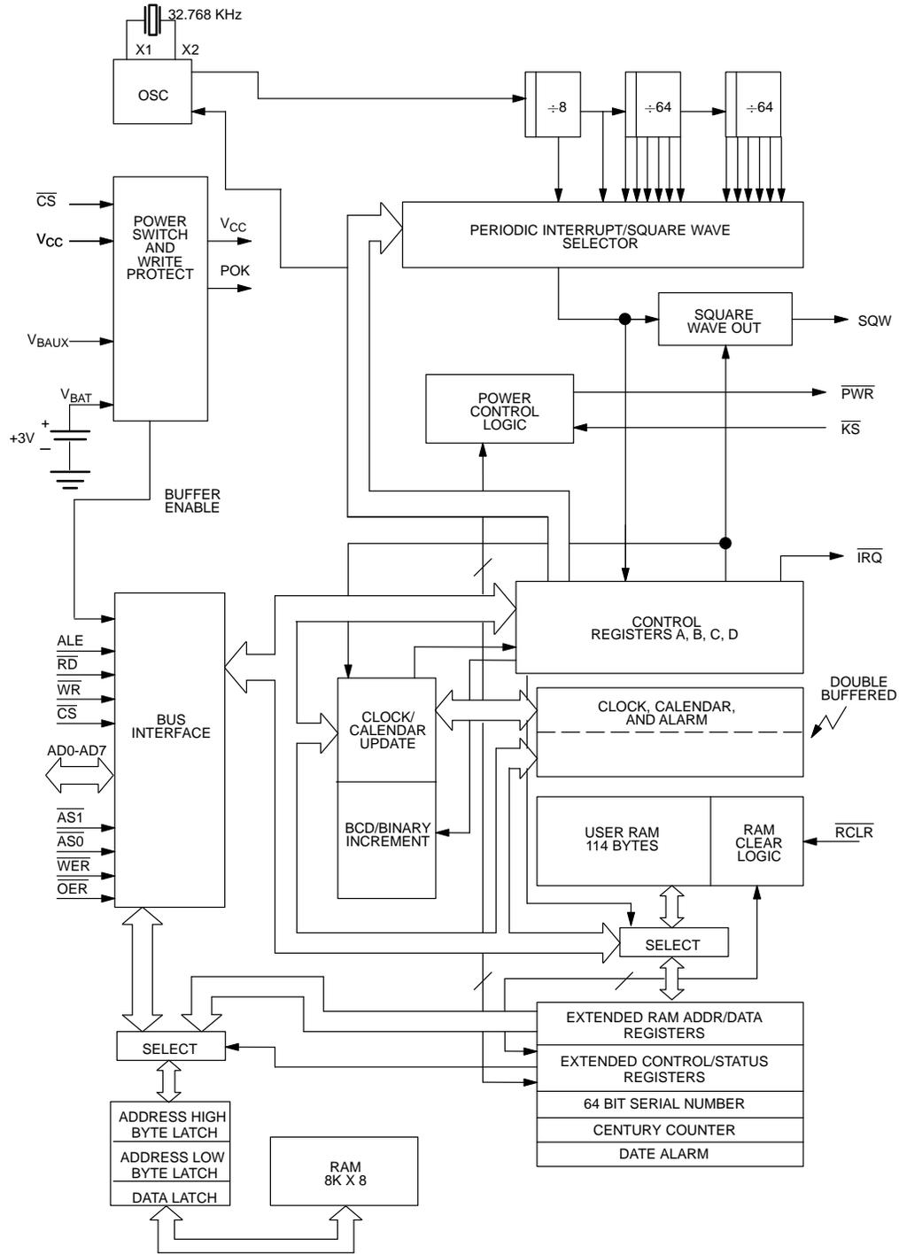
**ALE (RTC Address Strobe Input)** - A pulse on the address strobe pin serves to demultiplex the bus. The falling edge of ALE causes the RTC address to be latched within the DS1585/DS1587.
