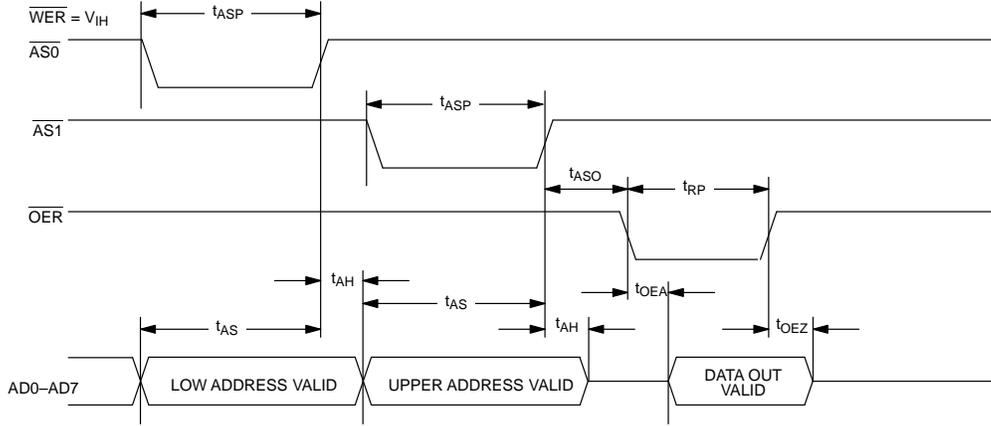
**BUS TIMING FOR WRITE CYCLE TO 8K X 8 SRAM**
