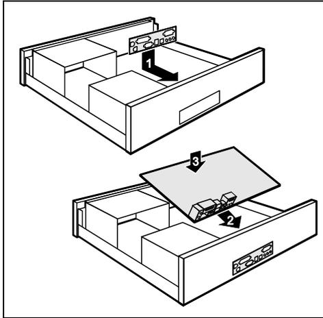
Ê Should no suitable connection field be provided in the case, then you must install the connection field (1) provided.
