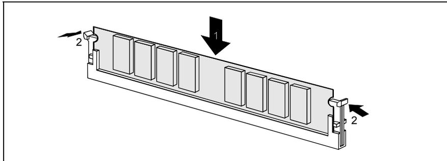
Ê Push the holders on each side of the memory compartment outwards.
