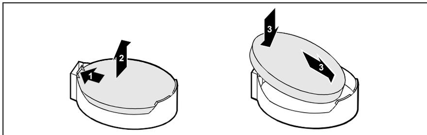
Ê Press the locking lug in the direction of the arrow; the battery jumps somewhat out of the holder (1).
