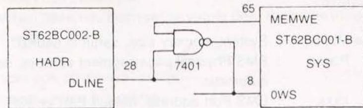
3. An additional circuit to be needed for 0 WAIT when DRAM is in state of READ or WRITE and when PROM is in state of READ:
