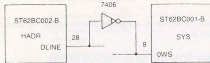
2. An additional circuit to be needed for 0 WAIT when DRAM is in state of READ:
