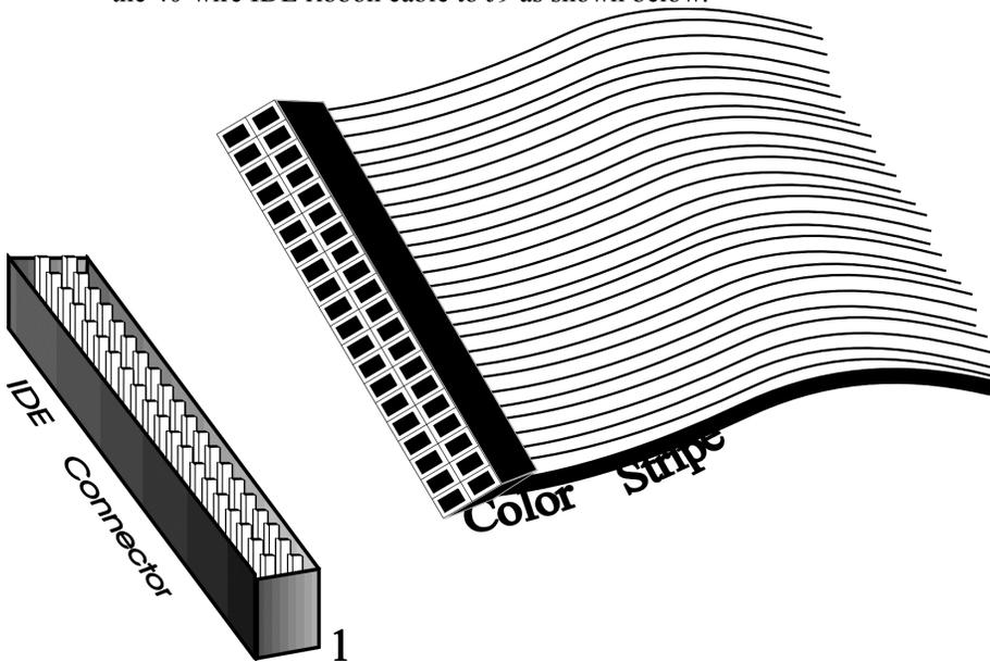
When you use the onboard IDE controller in conjunction with another hard drive controller, you must make sure that there are no conflicts in IRQ and I/O port addresses. The onboard IDE uses IRQ14 and I/O port addresses 01F0h – 01F7h. If there is a conflict, the IDE interface can be disabled via Peripheral Setup (see page 97). The J9 pinout is:
