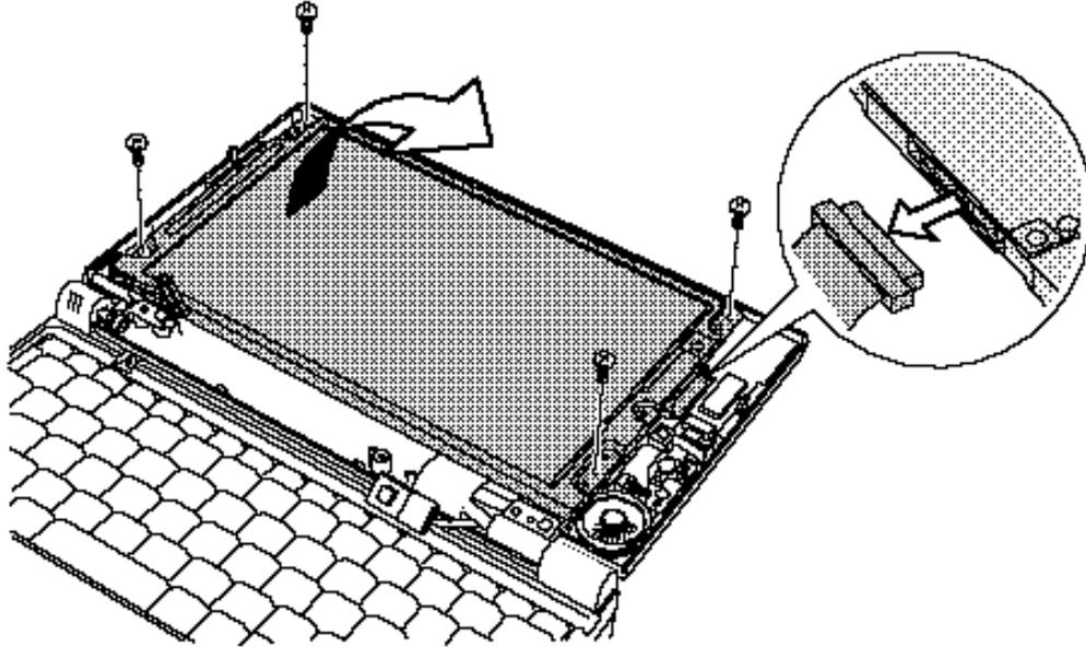
*Figure 4-20 LCD module removal*
