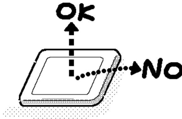
2. Be careful to align the holes at the four corners of the LCD module with the corresponding holes in its cover before securing the module with screws. Do not force the module into place, because stress can affect its performance.
