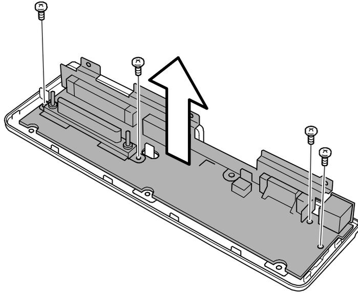
*Figure 4-32 Removing the I/O adapter board*
