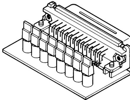
*Figure 2-2 Printer port LED*
