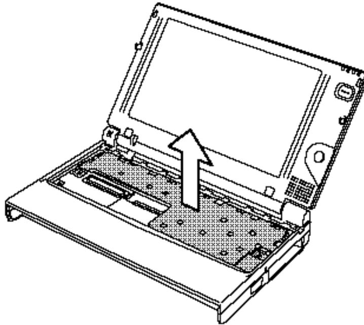
*Figure 4-8 Removing the metal cover*
