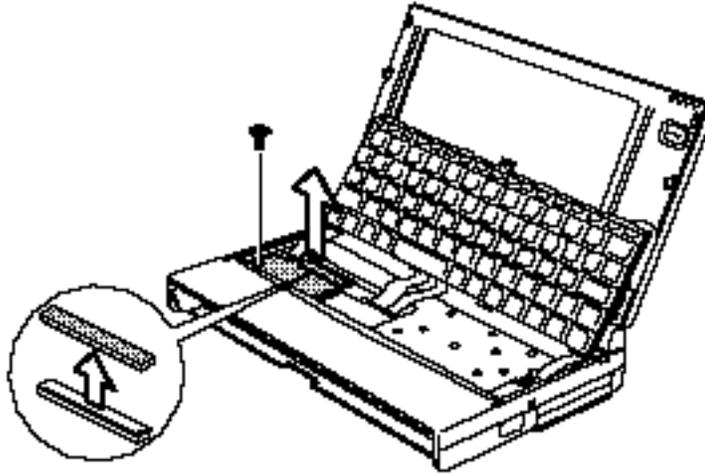
Figure 4-6 Removing the optional memory module
