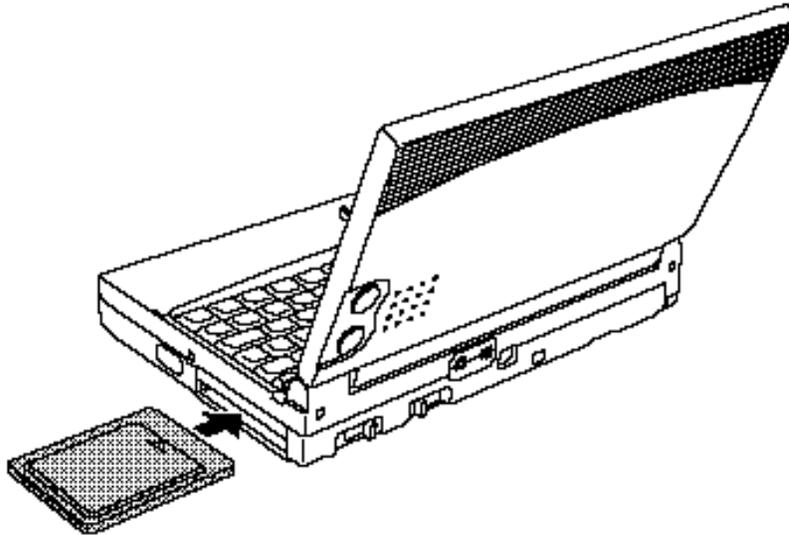
3. Insert the **PC card**. Carefully push it in place.
