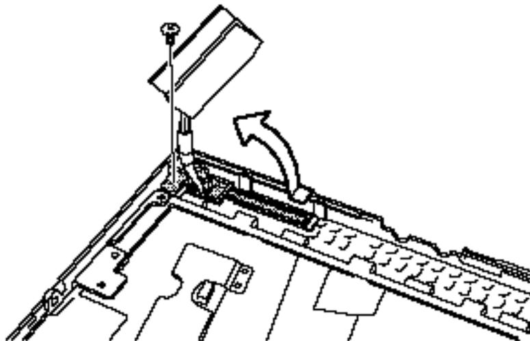
*Figure 4-28 Removing the LCD flexible cable*
