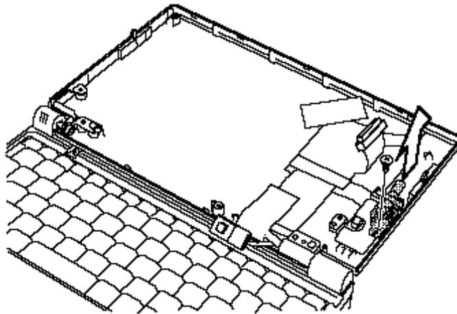
*Figure 4-23 Removing the AccuPoint board*
