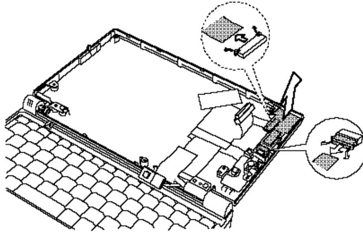
*Figure 4-22 Removing the power switch board*
