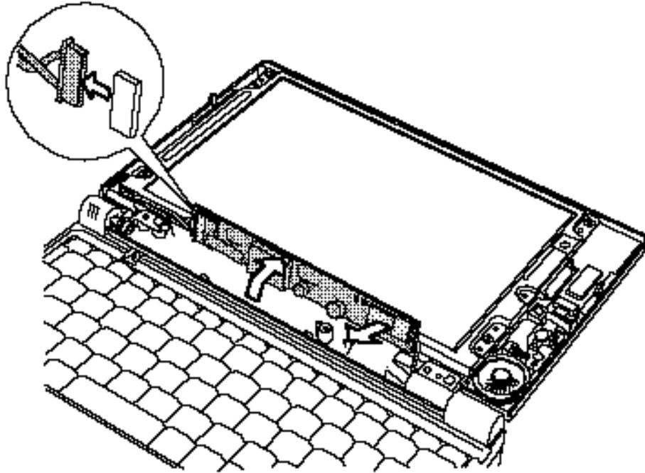
*Figure 4-19 Disconnecting the display cable*
