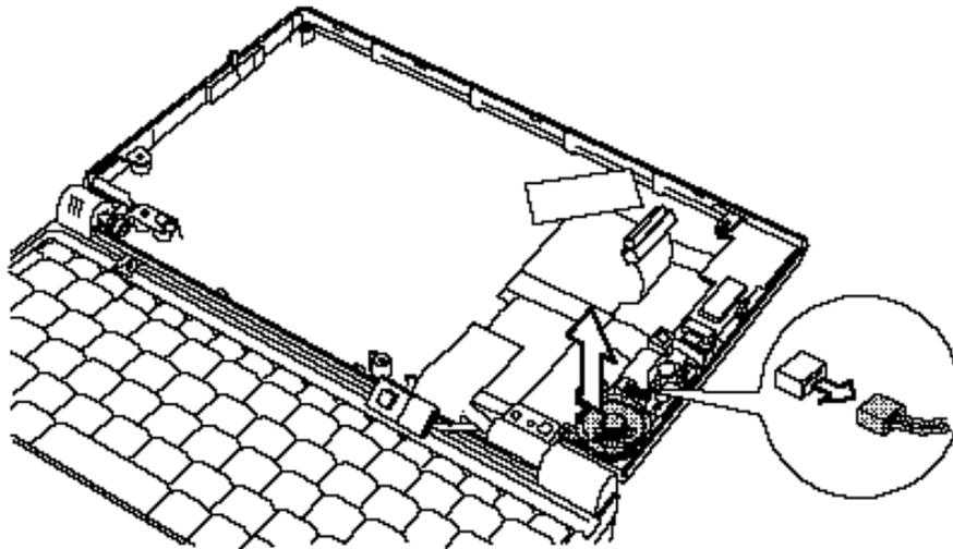
*Figure 4-21 Removing the speaker*
