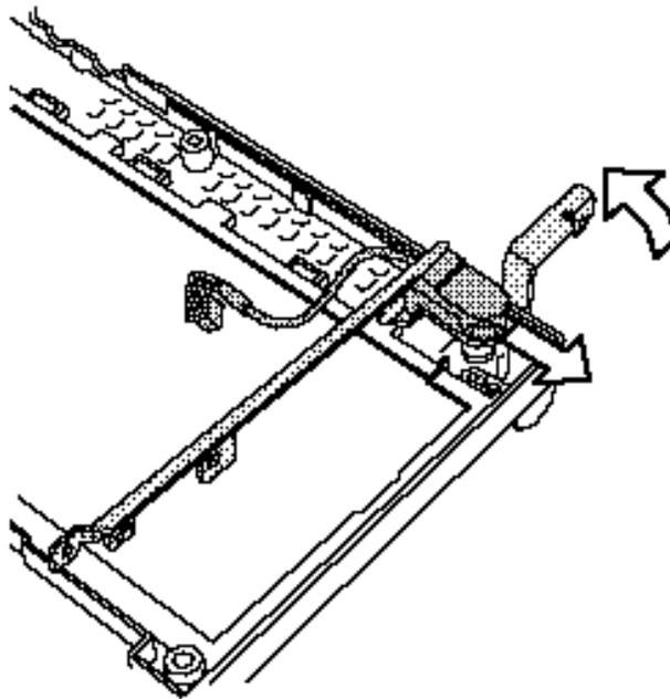
*Figure 4-27 Removing the left top cover brace and microphone*
