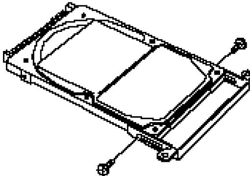
*Figure 4-3 Removing the HDD bracket*
