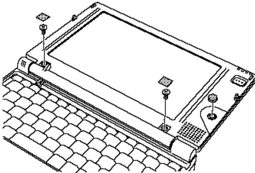
*Figure 4-16 Removing the mask seals*
