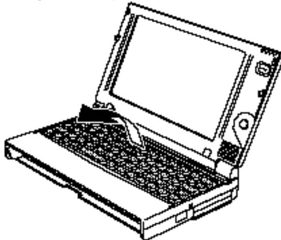
*Figure 4-5 Lifting up the keyboard*
