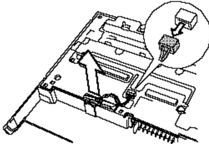
*Figure 4-12 RTC battery removal*
