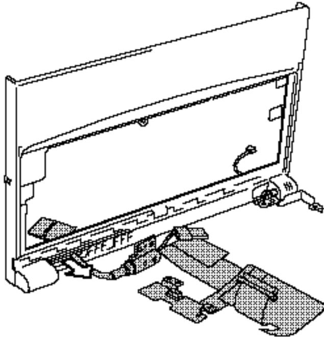
*Figure 4-29 Removing the LCD cable*
