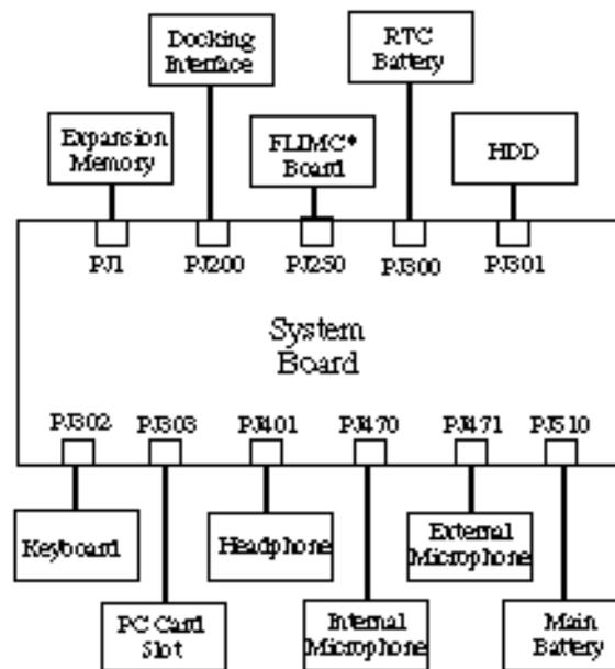
Figure 1-2 System unit configuration
