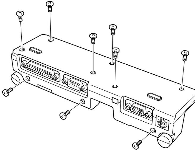
*Figure 4-30 Removing nine screws*
