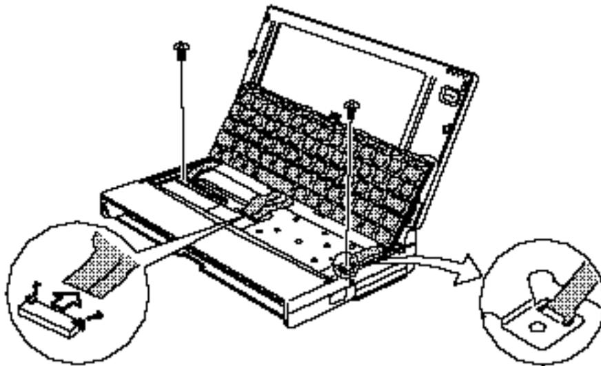
*Figure 4-7 Removing the keyboard*
