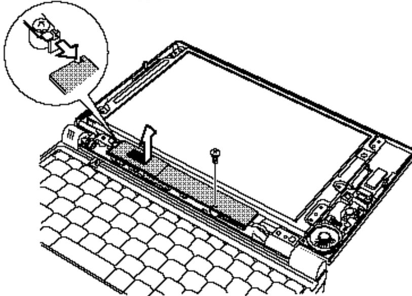
*Figure 4-18 Removing the FL inverter board*
