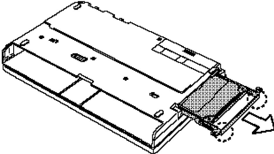
*Figure 4-2 Removing the HDD*
