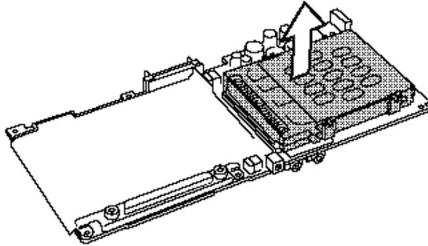
*Figure 4-15 Removing the PC card slot*
