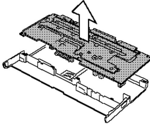
*Figure 4-13 Removing the system board*
