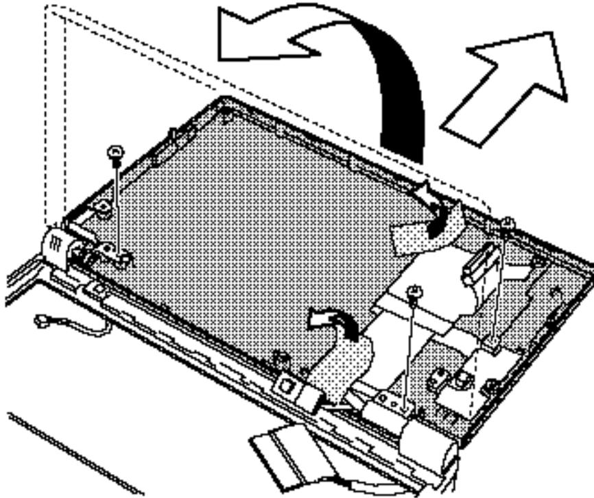
*Figure 4-24 Removing the LCD module*
