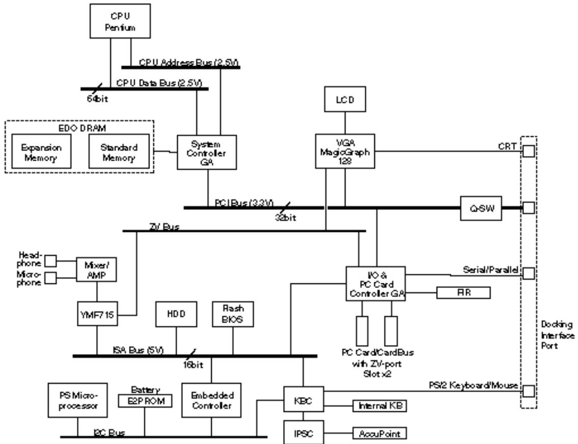
Figure 1-3 System unit block diagram
