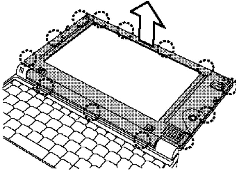
*Figure 4-17 Removing the display mask*
