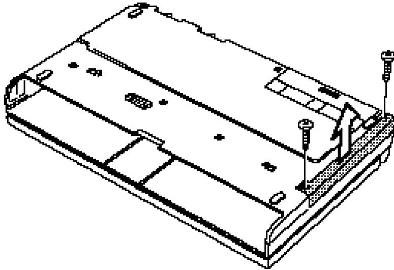
*Figure 4-1 Removing the HDD cover*
