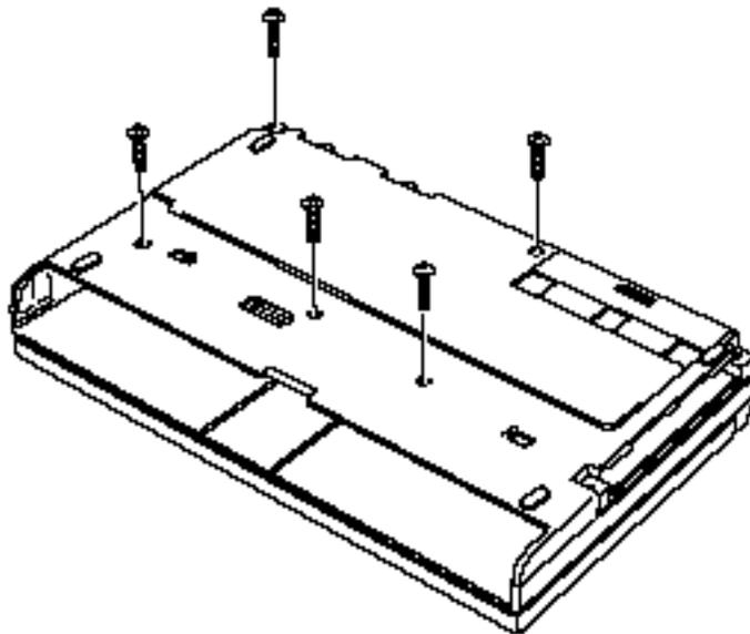
*Figure 4-10 Removing five screws*
