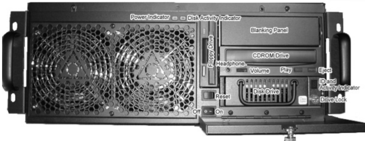
Figure 10-1 The Power Switch is the lowest of the two black switches. The reset switch is the black switch above the power switch.
