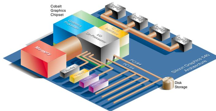
Figure 1-1. An Architecture Optimized for Visual Computing
