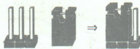
Figure 2 - 1 Jumper with Pins Shorted
