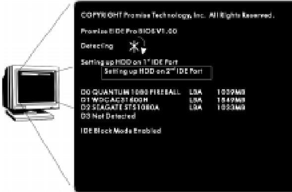
The EIDEPRO BIOS enables LBA if it reads that the Mainboard BIOS is set for Drive Type 1. Then it autosenses IDE hard disks on the Secondary (J2) IDE controller and automatically sets up LBA parameters.
