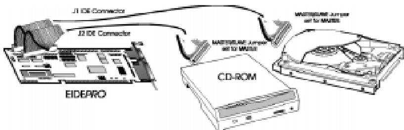
**Note:** If using an IDE CD-ROM and IDE disk drive together on the J2 IDE channel, remember to set the IDE disk drive as Master and the IDE CD-ROM as Slave (see manufacturer's manual).
