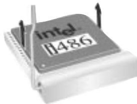
Figure 3.4 Removing the 486 from a ZIF Socket with a Sidebar
