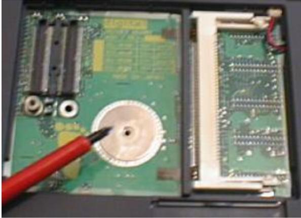
Undo the screw that is revealed, which holds down the keyboard, which also acts as the heatsink.
