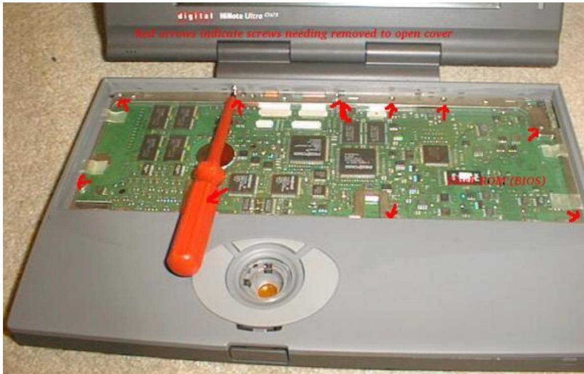
>Around the system board you will find the remaining screws holding the
