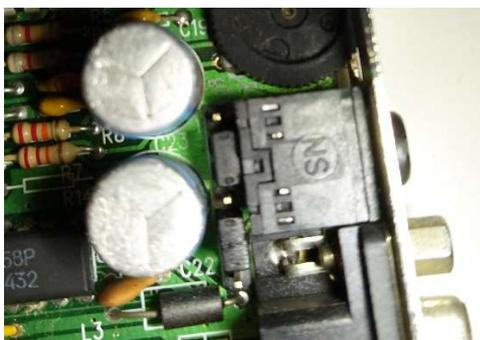
If you have powered speakers, configure as shown (each jumper one position in towards the centre) to bypass the onboard amp and volume control.
