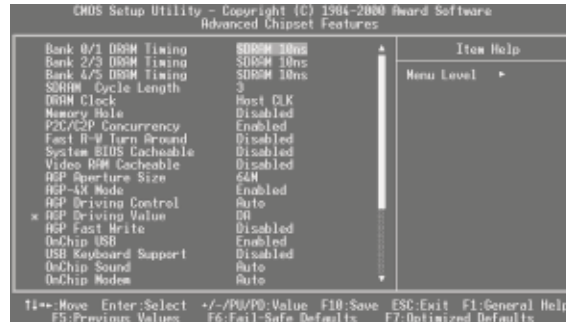
Figure-5 Advanced Chipset Features Setup Menu
